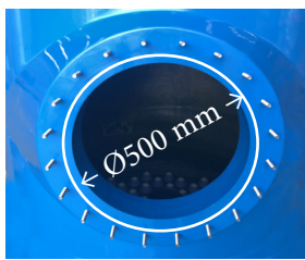
Upgrade from access manhole Ø 420 mm to Ø 500 mm
