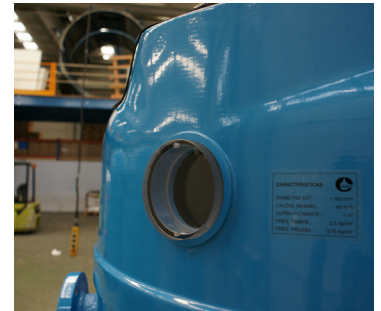
100% full vision inside: Methacrylate sightglasses
