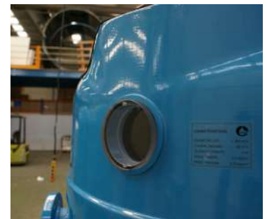
100% full vision inside: Methacrylate sightglasses
