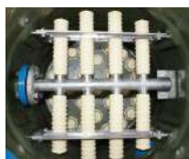
Stainless Steel beams with PP arms
