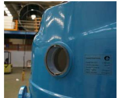
100% full vision inside: Methacrylate sightglasses
