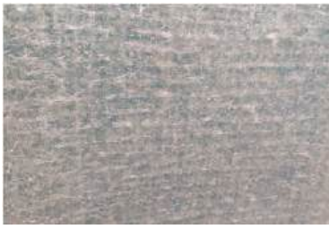
Manually laminated hand lay-up polyester resin fiberglass to controlled thickness.
