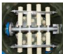
Stainless Steel beams with PP arms
