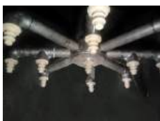
Stainless Steel star with PP nozzles
